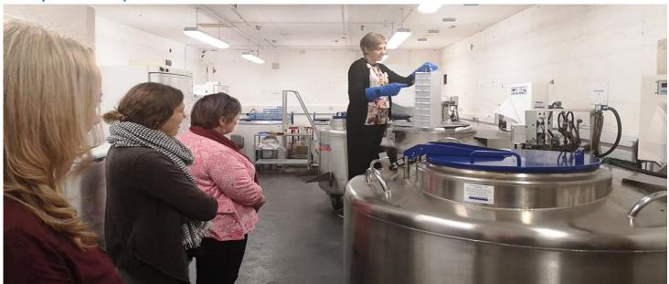
Fragile biological samples are preserved in these tanks by cooling them to very low temperatures using liquid nitrogen
